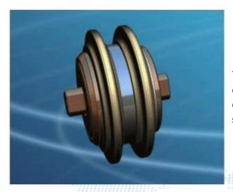
The double disc cutter is installed on the front and edge of the cutter head, and is mostly used for crushing soft rock with low uniaxial compressive strength (UCS≥70Mpa).
